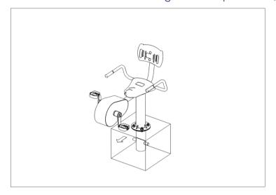
V. Make sure the machine is vertical to the ground and fix well, pour the concrete, and block the space.
