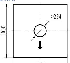
II. Please make sure the centre point of circular, square must comply with the centre point of installation position of each machine in the project diagram.
