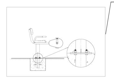
Please be attention: the top of flange must be at the same level or above of ground during process of pouring concrete.
