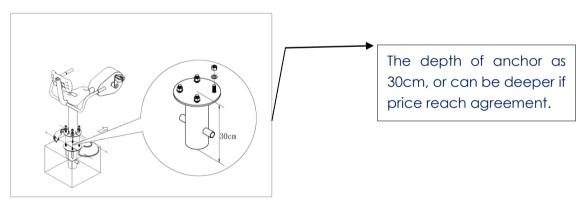
Based on the project diagram, make a circular mark at the center of installation site for each machine, and draw an installation direction by making square mark with sides of 1000mm outside the circular. And dig an embedded hole (with size of Ø234\*300mm) at each marked position of ground;
